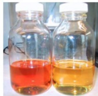
Illu. 1, EHC fluid before and after conditioning
