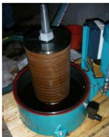
Illustration 9, Used fine filter insert. Illu.10, Used ion exchange insert.
