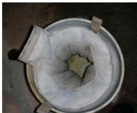
Illustration 9, Used fine filter insert. Illu.10, Used ion exchange insert.
