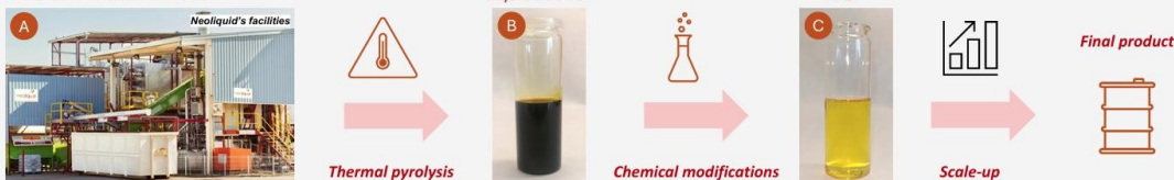
Figure 4. Pao production process ((A) Neoliquid's facilities, (B) liquid fraction obtained from thermal pyrolysis & (C) PAO obtained from the chemical transformation of the liquid fraction).
