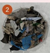
Figure 2 & 3. Waste used in the thermal pyrolysis process ((1) plastic waste, (2) plastic & biomass waste).
